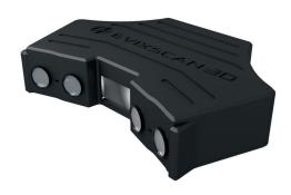
The eviXscan 3D Quadro+ scanner is distinguished by two scanning ranges that allow to measure the geometry of both large objects (up to 130 cm) and precise elements (from 5 cm). Changing the scanning range is done in the software, so recalibration is not required. Compared to the previous version, the Quadro+ scanner has been equipped with cameras with much higher resolution, which translates into greater measurement accuracy.
