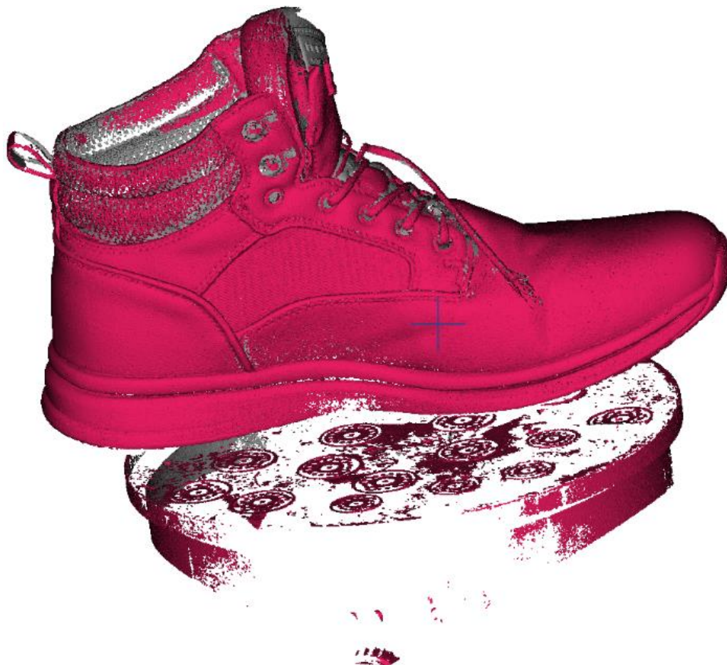
Figure 282. Scanning without the plane cut-off option enabled
