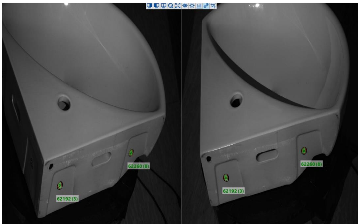
Figure 212. Preview of the detected 2D marker that can be converted to 3D marker
