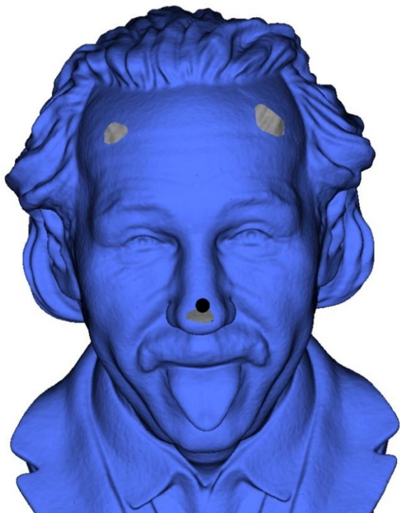
Figure 446. The mesh before filling the hole
