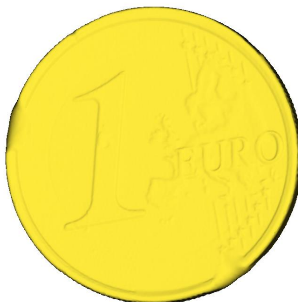
Figure 457. The mesh after using fill holes densely algorithm
