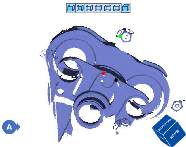
Figure 386. Marked points on the reference scan
