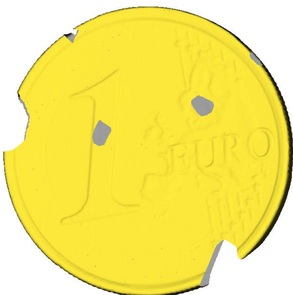
Figure 456. The mesh before using fill holes densely algorithm
